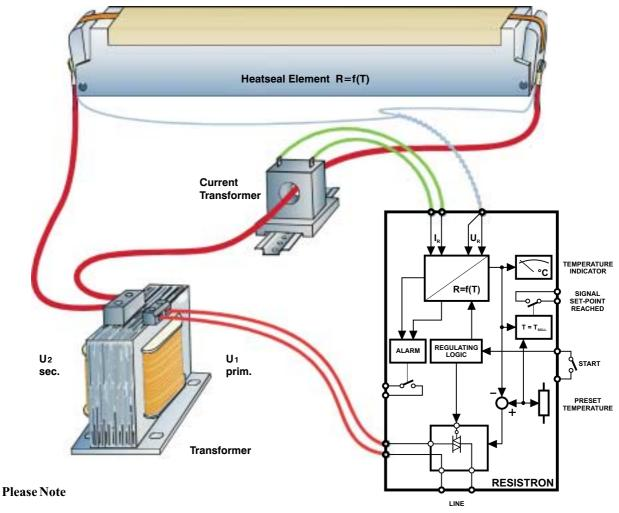
The **RESISTRON temperature controllers** are important components for modern machines with higher speeds. The technical possibilities offered by this control system however, can only be achieved by optimizing the **complete system**.
