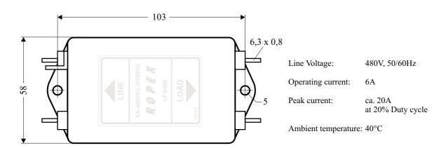
It is admissible to operate several RES-Control-circuits with one filter as far as the total current does not exceed the filter current.
