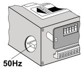
Position the Jumper (13) to select 50 or 60Hz frequency
